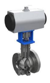
ZJHV V-notch ball valve is consist of Pneumatic piston actuator, electric actuator and V-notch ball valve components. It has the features of compact construction, light weight, small volume, convenient maintains, unimpeded flow passage, low flow resistance, perfect sealing and low leakage. It is applicable for controlling high viscosity medium with fiber and granule and for many industries such as electric power, chemical industry, paper-making and light industry, etc.
