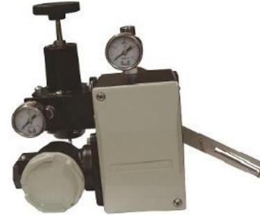
HEP15 / 16/17 Single acting electric-pneumatic valve positioner is the main accessory of CV3000 series regulating valve, which is used with pneumatic film actuator. This series of locators using force balance principle, the regulator output of the electrical signal into the control valve to change the gas signal to ensure that the regulator valve regulator output signal quickly and correctly positioned; also can change the flow characteristics of the valve Or the type
