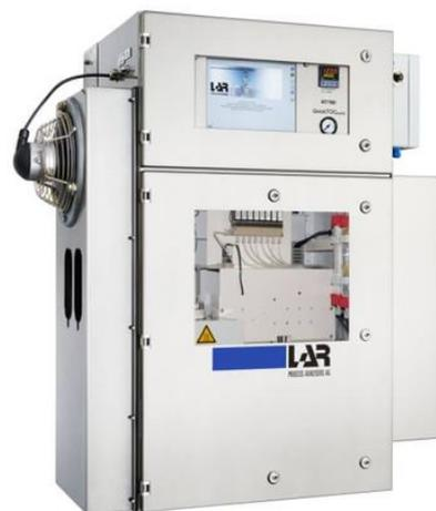
LAR's online total organic carbon analyser determines the TOC in less than three minutes and thus, allows the operators to take fast countermeasures in case of water pollution.
